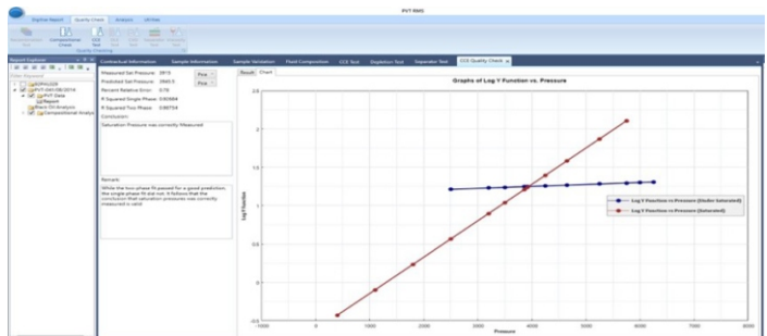
CCE Quality Check Log Y Function vs Pressure (Saturation Pressure Validation)
